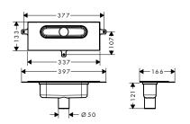
Water seal height: 50 mm Minimum height: 0 mm Drainage capacity siphon: 42 l/min
