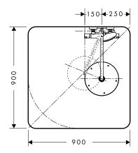
Showerpipes can easily be installed on the front or long side of the bath, according to the positions of the water connections. The overhead shower can also be aligned individually.
